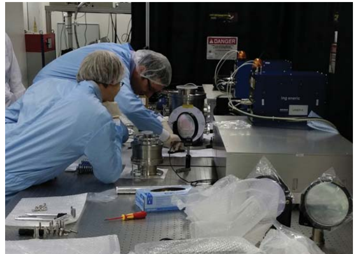
Dr. Paul Mason and Dr. Andrew Lintern from STFC Rutherford Appleton Laboratory are installing the Yb:YAG slabs inside the amplifier head. The slabs are cooled by a Helium closed-loop at temperature of 150 K.
