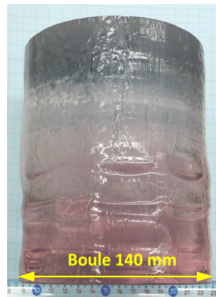
Large monocrystals developed in cooperation with Czech industry within the ELI-Beamlines project. The core-free Yb doped YAG crystals with up to 5' in diameter and 6' long are the largest of its kind in the world.
