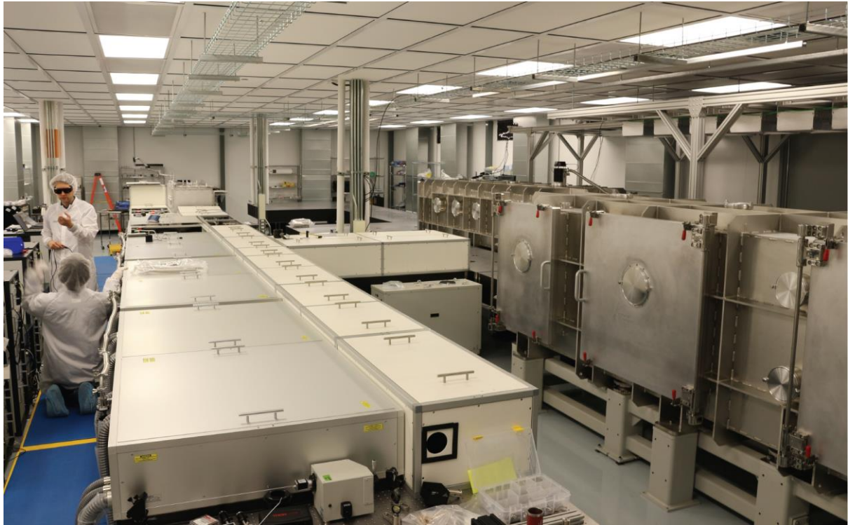
Laser L4 chain in the development laboratories at National Energetics (USA), with the front end of the system seen in the forefront.
