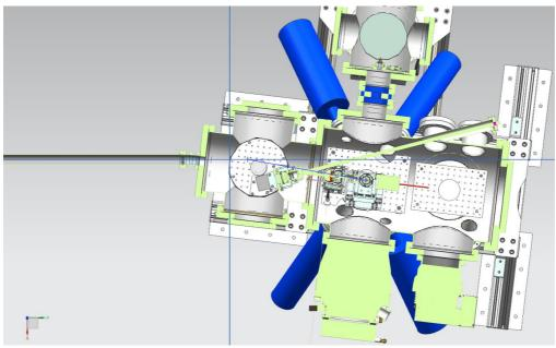
Model of the MAC station with two different focal geometries. One using a 10 degrees grazing incidence ellipsoidal mirror (current geometry) and another utilizing a 11 degrees angle of incidence Off Axis Parabola (optional geometry).
