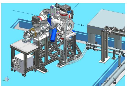
Model of the MAC station on the beamline location. In this image the station is equipped with the aerosol injector mounted from the top of the main chamber and a cluster source with a cryo-cooled Even Lavie nozzle (under development) mounted from the side.
