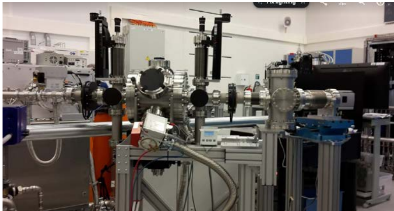
Fig: ELIps set up for VUV transmission and reflection on the HHG beamline in the E1 experimental hall.
