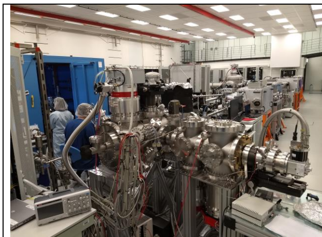
Fig 2. The MAC end station with cryo-cooled cluster source during testing in the E1 experimental hall.
